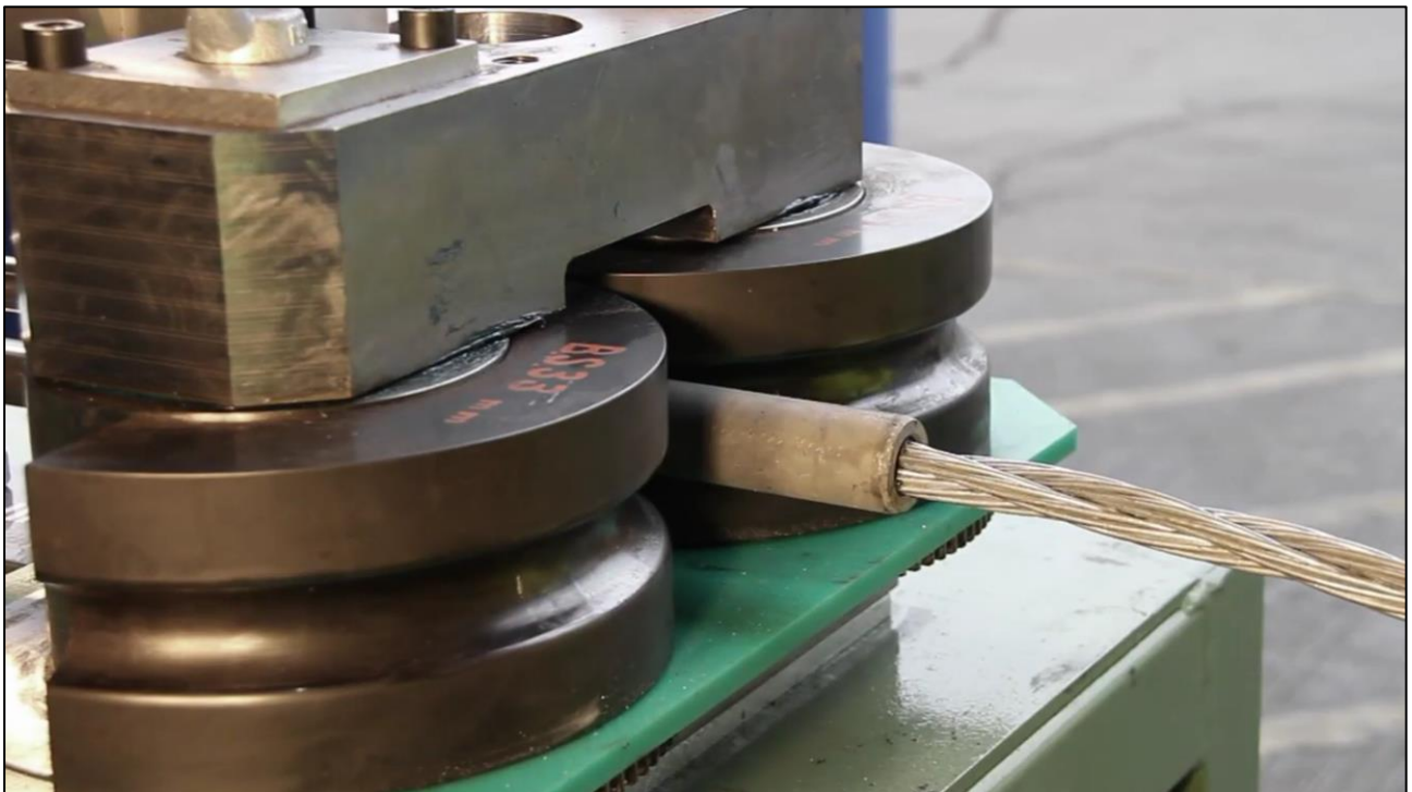
Figure 8: Insert wire rope into fitting to the required depth of 120mm
