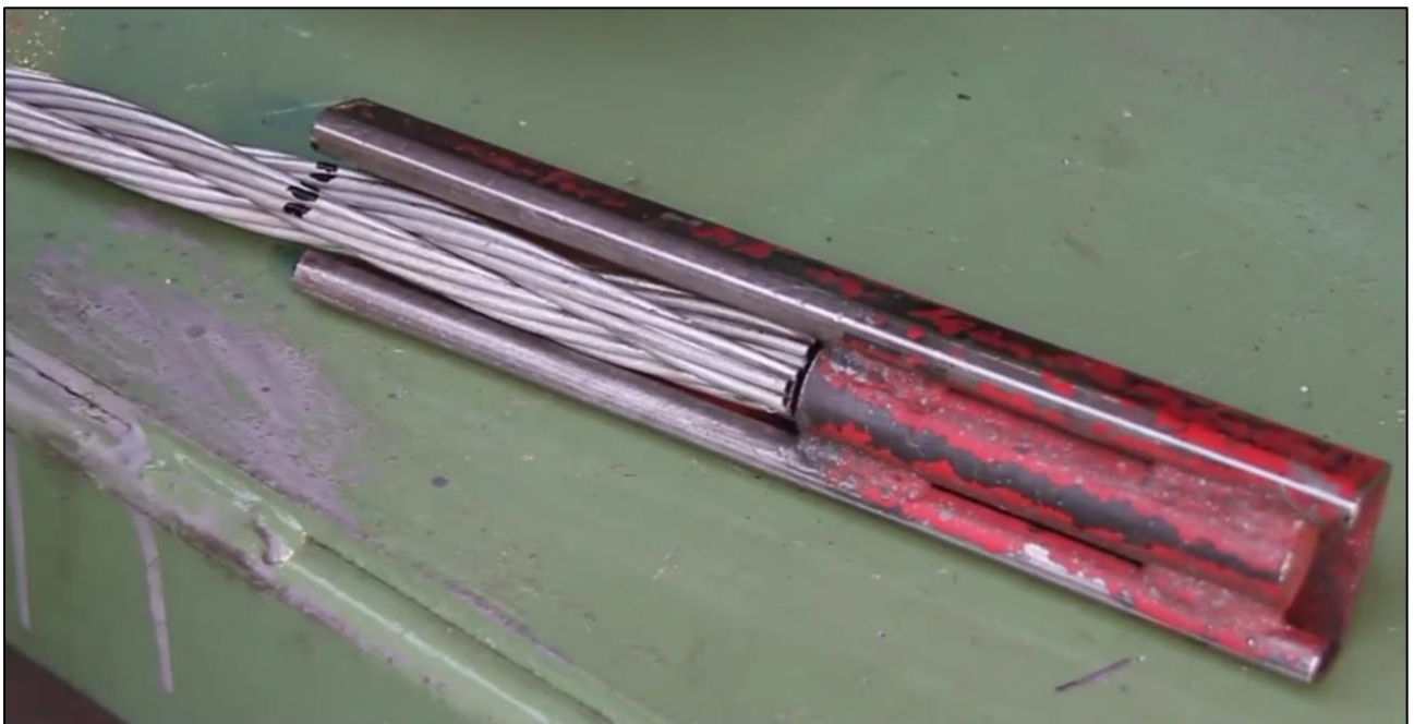
Figure 6: Swaging depth of 120mm
