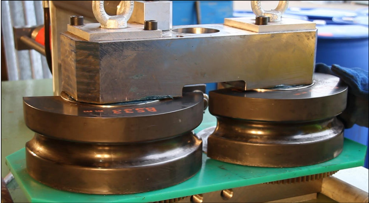
Figure 3: Swager dies starting position - front view
