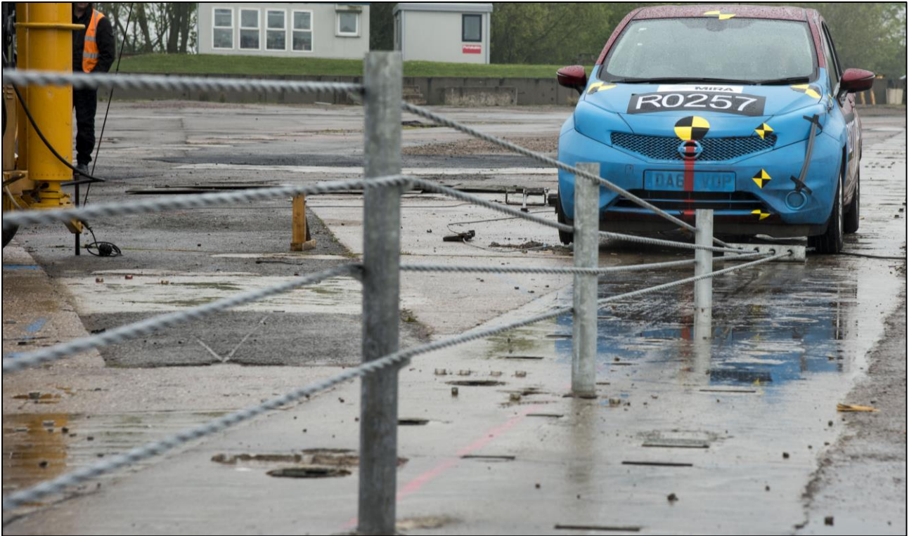
Figure 13: Cable Weave at Terminal
